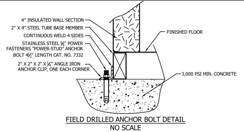
THIS DRAWING IS FOR REFERENCE PURPOSES ONLY. PAR-KUT BUILDINGS MUST BE SECURELY ANCHORED IN PLACE AND ELECTRICAL SYSTEM MUST BE PROPERLY GROUNDED. ADEQUATE SIZED ANCHOR BOLTS SHALL BE USED. THE SIZE AND DEPTH OF THE ANCHORS SHOULD BE OF SUFFICIENT DESIGN TO WITHSTAND THE HIGHEST RECORDED WIND SPEEDS/SEISMIC DESIGN CATEGORY IN THE AREA OF INSTALLATION. CONSULT A PROFESSIONAL ENGINEER FAMILIAR WITH THE WEATHER CONDITIONS IN THE AREA.
