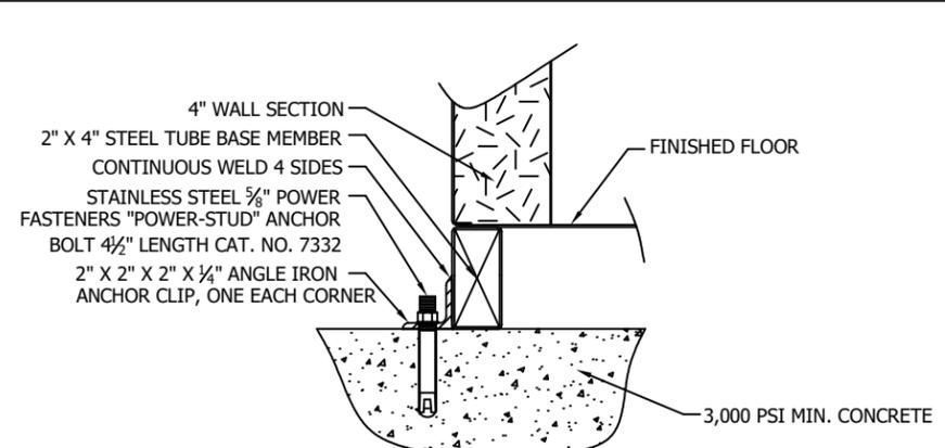
**FIELD DRILLED ANCHOR BOLT DETAIL**
