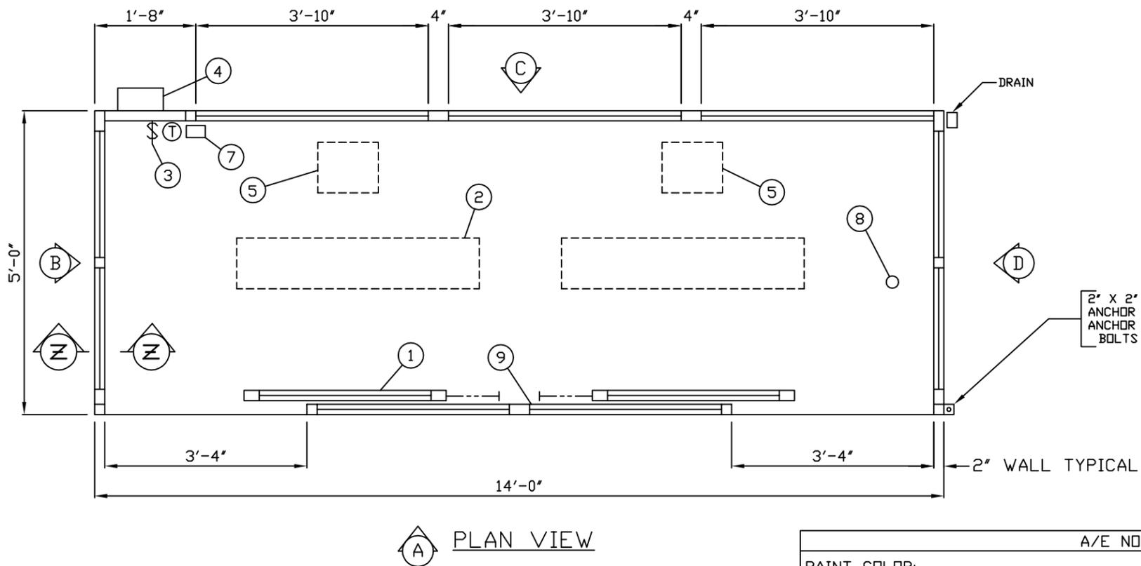
2" X 2" ANCHOR CLIP WELDED TO BASE WITH 3/4" ANCHOR BOLT HOLE, 4-REQ'D., ONE EACH CORNER. ANCHOR BOOTH AFTER FINAL LOCATION. ANCHOR BOLTS NOT INCLUDED.
