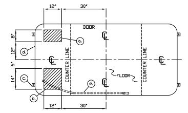
NOTE: PROVIDE 120/208V. 10-3 WIRE SERVICE WITH GROUND. SERVICE ENTRANCE/ANCHOR BOLT LAYOUT
