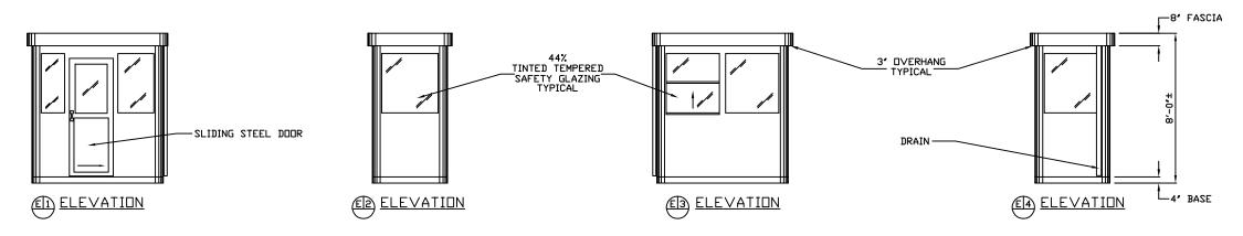
4" INSULATION 14 GA. GALV. STEEL ROOF, CANOPY, & CEILING-ALUMINUM INTERIOR GLAZING STOP FLOOR TO CEILING 6'-8" FLOOR TO SILL 3'-4" FLOOR TO COUNTER 2'-8" FLUDRESCENT LIGHT FIXTURE-SAFETY GLAZING PAINTED STEEL EXTERIOR WINDOW FRAME 14 GA. PAINTED GALV. STEEL COUNTER STORAGE DRAWER DUPLEX DUTLET-14 GA. GALV. STEEL DUTER PANEL HEATER 2" INSULATION-18 GA. GALV. STEEL INNER PANEL-12 GA. GALV. 4-WAY DIAMOND PLATE STEEL FLOOR (PAINTED) 2" X 4" GALV. STEEL TUBE BASE-
