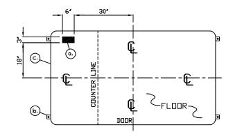
NOTE: PROVIDE 120/240V. 10-3 WIRE SERVICE WITH GROUND. SERVICE ENTRANCE/ANCHOR BOLT LAYOUT
