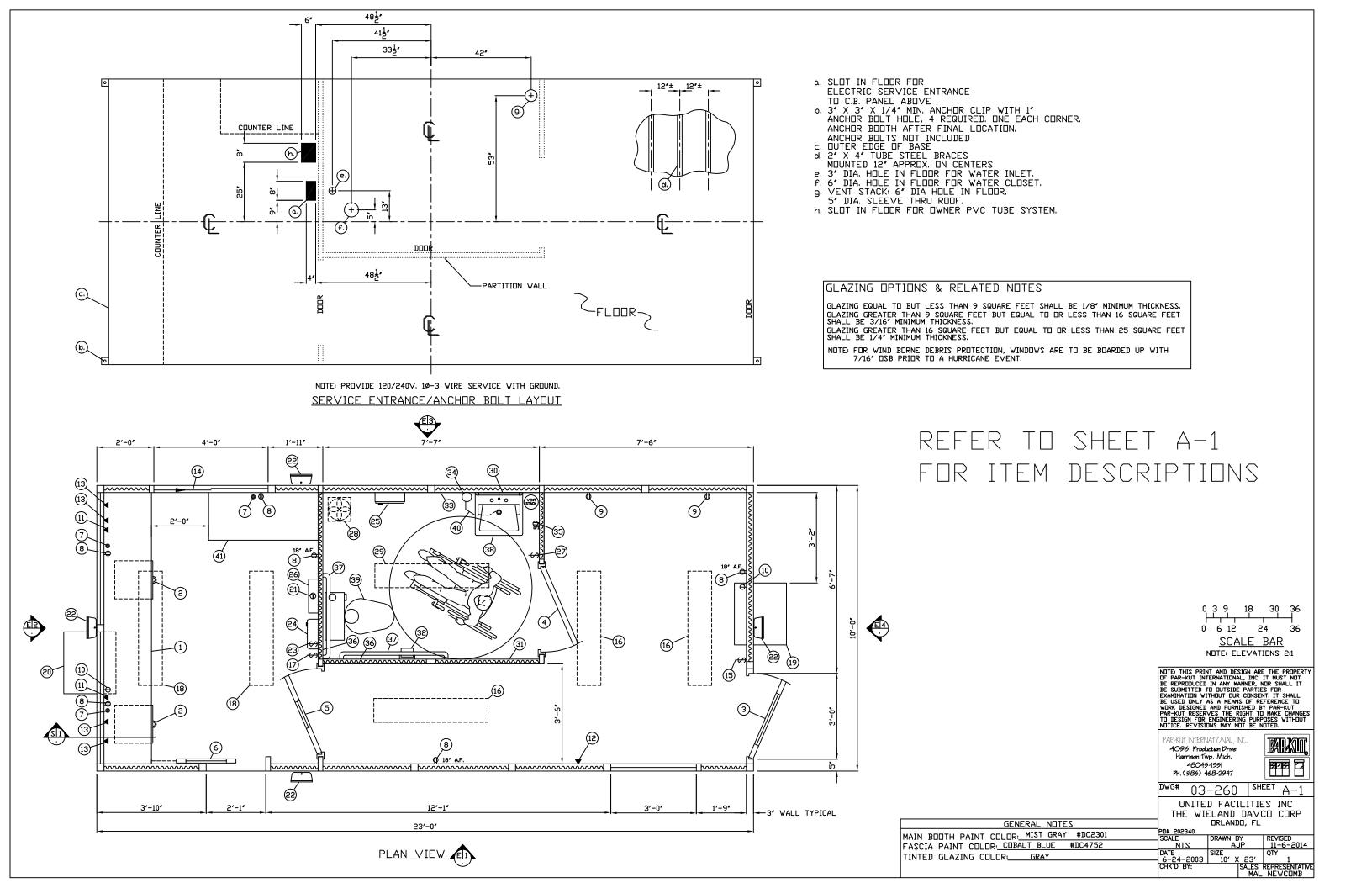
COUNTER- 20" DEEP PAINTED GALVANIZED STEEL MOUNTED 32" ABOVE FLOOR. PAINTED STORAGE DRAWER BENEATH COUNTER, 2-REQ'D. DOOR- 36" WIDE, SWINGING STEEL WITH WEATHER-STRIPPING, BALL BEARING BUTTS, SAFETY GLAZING, HYDRAULIC CLOSER, LEVER HANDLE LOCK, & HARDWARE. PRIVACY DOOR- 36" WIDE, SWINGING STEEL WITH LEVER HANDLE LOCK.
