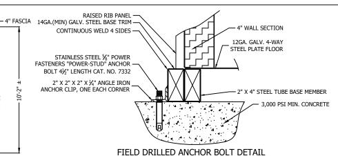
THIS DRAWING IS FOR REFERENCE PURPOSES ONLY. PAR-KUT BUILDINGS MUST BE SECURELY ANCHORED IN PLACE AND MUST BE PROPERLY GROUNDED. ADEQUATE SIZED ANCHOR BOLTS SHALL BE USED. THE SIZE AND DEPTH OF THE ANCHORS SHOULD BE OF SUFFICIENT DESIGN TO WITHSTAND THE HIGHEST RECORDED WIND SPEEDS/SEISMIC DESIGN CATEGORY IN THE AREA OF INSTALLATION. CONSULT A PROFESSIONAL
