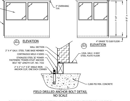
THIS DRAWING IS FOR REFERENCE PURPOSES ONLY. PAR-KUT BUILDINGS MUST BE <u>SECURELY</u> ANCHORED IN PLACE AND ELECTRICAL SYSTEM MUST BE PROPERLY <u>GROUNDED</u>. ADEQUATE SIZED ANCHOR BOLTS SHALL BE USED. THE SIZE AND DEPTH OF THE ANCHORS SHOULD BE OF SUFFICIENT DESIGN TO WITHSTAND THE HIGHEST RECORDED WIND SPEEDS/SEISMIC DESIGN CATEGORY IN THE AREA OF INSTALLATION. CONSULT A PROFESSIONAL ENGINEER FAMILIAR WITH THE WEATHER CONDITIONS IN THE AREA.
